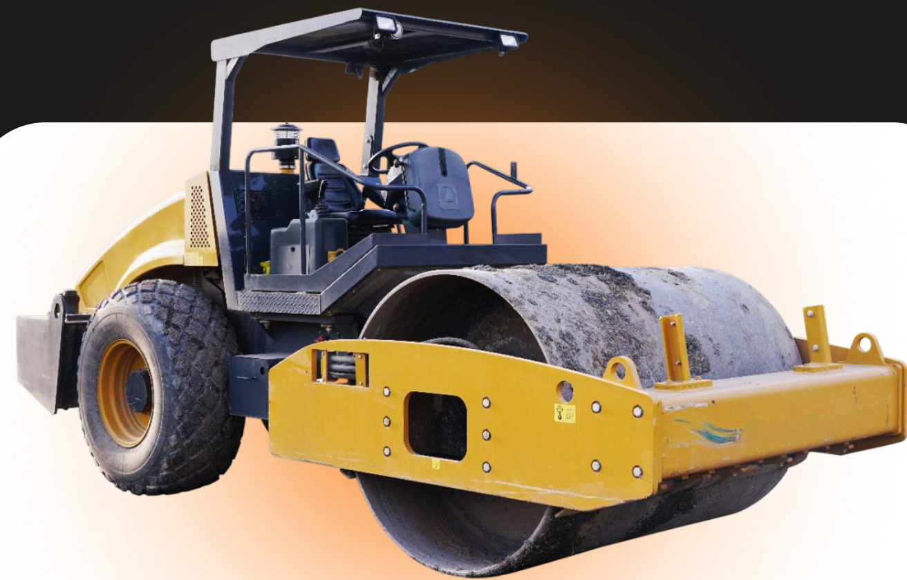
STATIC ROLLERS for initial compaction
